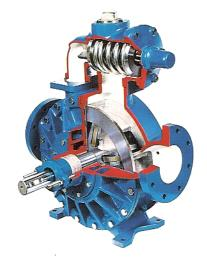
Model MLN - Ideal for handling thin to highly viscous fluids such as oils, asphalts, molasses and adhesives. The MLN features internal self-lubricating carbon sleeve bearings and PTFE-impregnated shaft packing. Options include Blackmer or commercial single or double mechanical seals.
