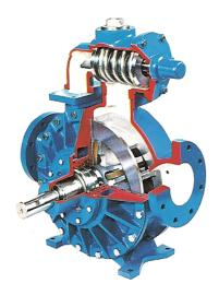
Model MLX - Designed for handling all types of liquids from light non-lubricating to viscous abrasive slurries and waste oils. The hub assembly in this model features external grease-lubricated spherical roller bearings and can be fitted with a wide selection of Blackmer mechanical seals. Two-piece threaded lock collars allow for vertical or horizontal pump mounting. Options include hardened or wear resistant internal components
